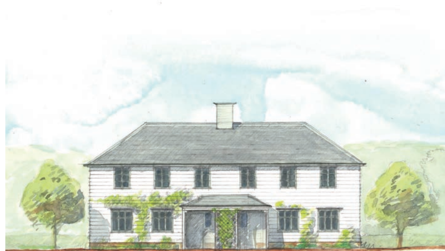
3 bedroom affordable house elevation – semi-detached with weatherboard
