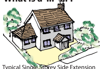
Typical Single Storey Side Extension Reduced Ridge Height
