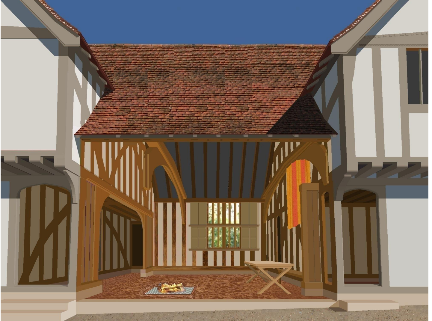
A reconstruction drawing by Tim Howson showing the medieval open hall of 4 Silver Street with its front wall omitted. The hall was open to the roof and heated by an open hearth, akin to a bonfire burning on its floor. Remarkably, part of the hearth was discovered beneath modern flooring alongside sherds of medieval cooking vessels.
