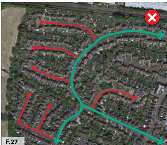
Figure 27: An example of a layout which is mainly dominated by cul-de-sacs encourages reliance on cars for local journeys and blocks pedestrian flow.
