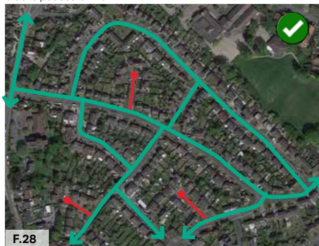
Figure 29: An example of a connected layout, with some cul-de-sacs, balances sustainability and improves the sense of a walkable neighbourhood.
